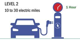
Requires installation of a 240-volt hardwired EV charger or the appropriate 240-volt receptacle for a plug-connected charger (installation must be completed by a qualified electrician). Some businesses offer Level 2 charging stations for their employees.
